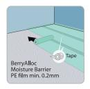
If you use the BerryAlloc moisture barrier separately (PE-film of 0.2 mm), you should always install it with an overlap of min. 20cm, taped and turned up against the walls. You can clean-cut the foil after the installation of the floor.
