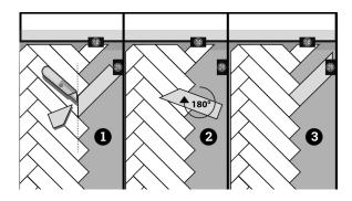
After installing the whole floor, the spacers must be removed so that the floor can expand and contract freely.
