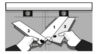
Now repeat the same method with plank (3) and (4). Plank (4) now serves as a stopper for plank (3). Fold down plank (3). Continue this process until you finish the center rows
