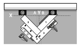
Work your way down. Do not forget to tap gently to perfectly engage the joint. Use a straight edge or additional reference line to ensure that the rows remain straight! Repeat this line with new rows.
