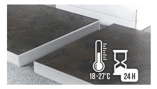
Installations in areas colder than recommended will influence the installation properties of Moduleo® Roots. The planks or tiles will be less flexible, cutting will be harder and small pieces difficult to cut out. The lower the temperature, the
